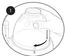
1 Place the Clear dome onto the Maker Station and twist clockwise until it locks tightly closed.
