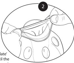
Start pumping and the balloon will 'inflate' within the clear dome. Keep pumping until the balloon fills the chamber. If the balloon doesn't inflate, check the clear dome is closed tight and the seal is clean.
